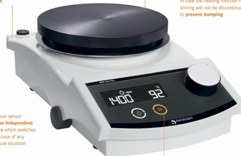
The temperature sensor consists of **two independent safety circuits** which switches off heating in case of any overtemperature situation
