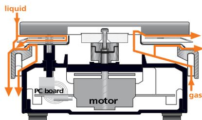
The hermetically-sealed housing that protects the PC board and the motor is marked in black. The way a liquid would take flowing down from the hotplate is marked in orange. As one can see, even if the liquid reaches the heat shields, it cannot ingress to the PC board and the
